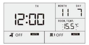
At normal mode screen, press [Frost ON/OFF] button one time to activate this function, denoted by the display frost symbol. Press [Frost ON/OFF] button again to deactivate, and the frost symbol will disappear.
