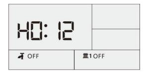
Press and hold [HOLIDAY ON/OFF] button for 3seconds to deactivate, when the holiday mode is activated. The programmer returns to normal mode.
