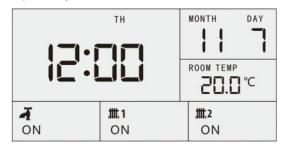
Operating mode: HW:ON C1:ON C2:ON
