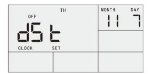
Daylight saving time is set to OFF DST symbol disappears.
