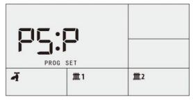
Fully Pumped and Controlled System (P). Central Heating and Hot Water can be operated independently.
