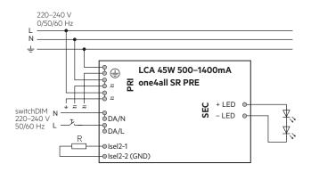
Device with loop through wiring function.
