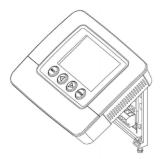
Tighten the 2 captive screws on the underside of the unit.
