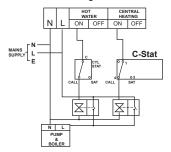
C-Stat replacing a conventional room thermostat on a fully pumped system with an existing programmer and two spring return valves with auxiliary switches
