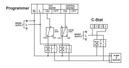
C-Stat controlling a secondary heating zone on a fully pumped system with existing programmer and two spring return valves with auxiliary switches
