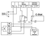
C-Stat replacing a conventional room thermostat on a fully pumped system with an existing programmer and 3 port mid-position valve.
