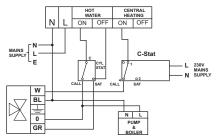
C-Stat replacing a conventional room thermostat on a fully pumped system with an existing programmer and 3 port mid-position valve.
