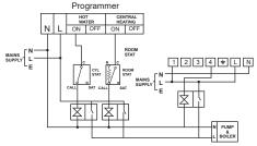
C-Stat controlling a secondary heating zone on a fully pumped system with existing programmer and two spring return valves with auxiliary switches.
