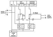
C-Stat replacing a conventional room thermostat on a fully pumped system with an existing programmer and two spring return valves with auxiliary switches All wiring diagrams are schematic and should be used for guidance only.
