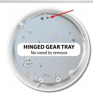
STEP 2 Loosen single gear tray screw
