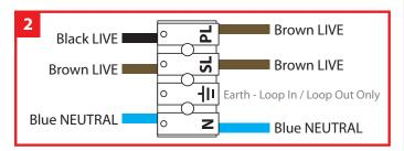
\*It is possible to convert a Maintained fitting into a Non-Maintained fitting - just remove the SL cable.
