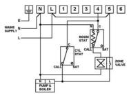
Fully Pumped System with RoomStat and two port spring return valve (with auxiliary switch) on Heating circuit
