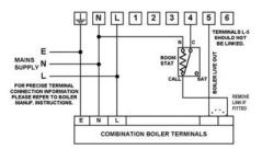
Typical combination boiler installation with RoomStat
