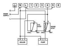
Gravity primary with pumped Heating via RoomStat and CylinderStat
