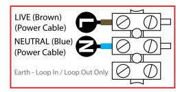
An Earth connection is not required for the operation of these Class II luminaires. The addition of the Earth terminal provides a loop-in/loop out facility which allows connectivity through to other Class I luminaires in the same lighting circuit.
