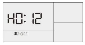
Press and hold [HOLIDAY ON/OFF] button for 3seconds to deactivate, when the holiday mode is activated. The programmer returns to normal mode.
