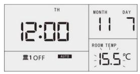
At normal mode screen, press [Frost ON/OFF] button one time to activate this function, denoted by the display frost symbol. Press [Frost ON/OFF] button again to deactivate, and the frost symbol `will disappear.
