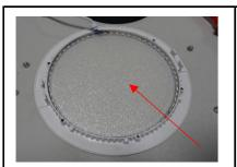
Lift out and remove Light Guide Plate and Diffuser
