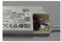
Remove LED output cable by pressing terminal release tabs
