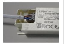
Remove Mains cable by pressing terminal release tabs
