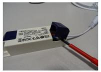
Remove both connection covers - lever with screwdriver
