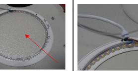
Diffuser removed - shows connector lead and LED Tape
