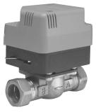
The Z222 valve with auxiliary switch has been designed to control the water circulation in fully pumped systems, which employ a single pump for both hot water and central heating circuits by allowing the flow to either or both circuits using separate valves.
